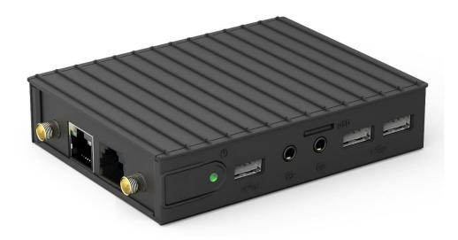
IOT-GATE-iMX7 is a powerful Industrial IoT Gateway PC based on the NXP i.MX7 processor designed for industrial control and monitoring.
